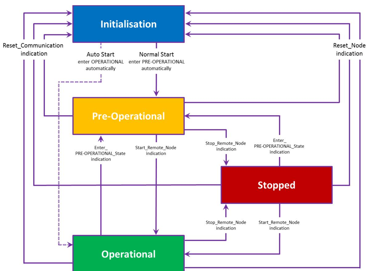
With the commands of an NMT master a certain one or all nodes in the network can be brought into different states. These commands are structured as follows:
