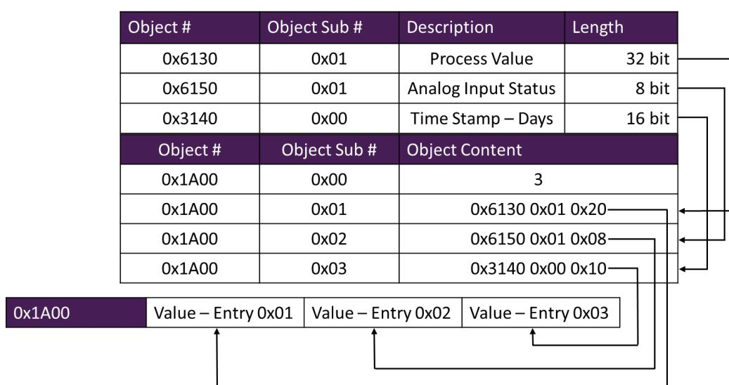
Both TPDOs' can be mapped with a valid number (the combined length of the mapped objects must not exceed the limit of 8 byte (64bit)) of process variables.
