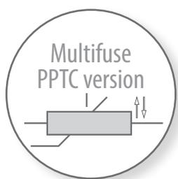
A multifuse (PPTC) works in a similar way like a PTC, which helps to overcome the challenges when switching high loads.
