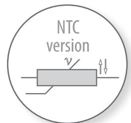
Our NTC version enables a temperature-controlled pressure switch action. By using a temperature depending component (NTC) the switch signal can get overruled until a certain temperature is reached. A typical application is in the filter monitoring of lubrication systems. With our NTC-Version we have integrated a cold start functionality in a mechanical pressure switch.
