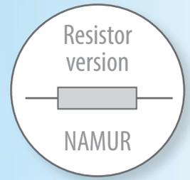
Our NAMUR resistor version is an essential solution for fail-safe applications, such as braking systems, fire extinguishing etc. By evaluating the resistance values you can always assure a correct connection and functionality of the switch – thus, this is the ideal solution for safety-relevant applications.
