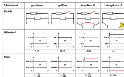
In the version with an additional resistor connection according to **NAMUR** SUCO offers a diagnostic function (fail-safe) with short-circuit and cable break detection. This version is of a special interest for safety systems as for example brake systems, hydrostatics steering systems or fire-fighting systems.
