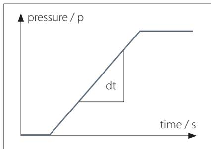
The maximum pressure change rate for mechanical pressure switches is 1,000 bar/s. For SUICO electronic pressure monitoring products the maximum pressure change rate can be up to 5,000 bar/s.
