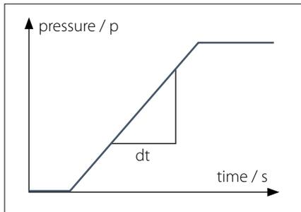
For SUICO electronic pressure monitoring products the maximum pressure change rate can be up to 5 bar/ms (5,000 bar/s).
